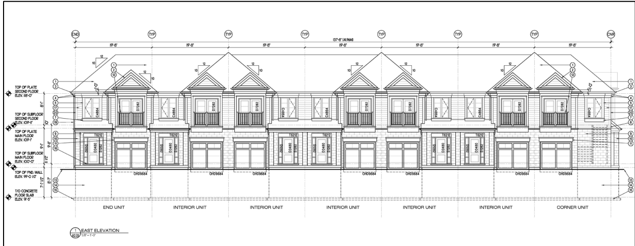
Figure 10 – Proposed Three-Storey Back-to-Back Townhouses Elevation (excerpt)
