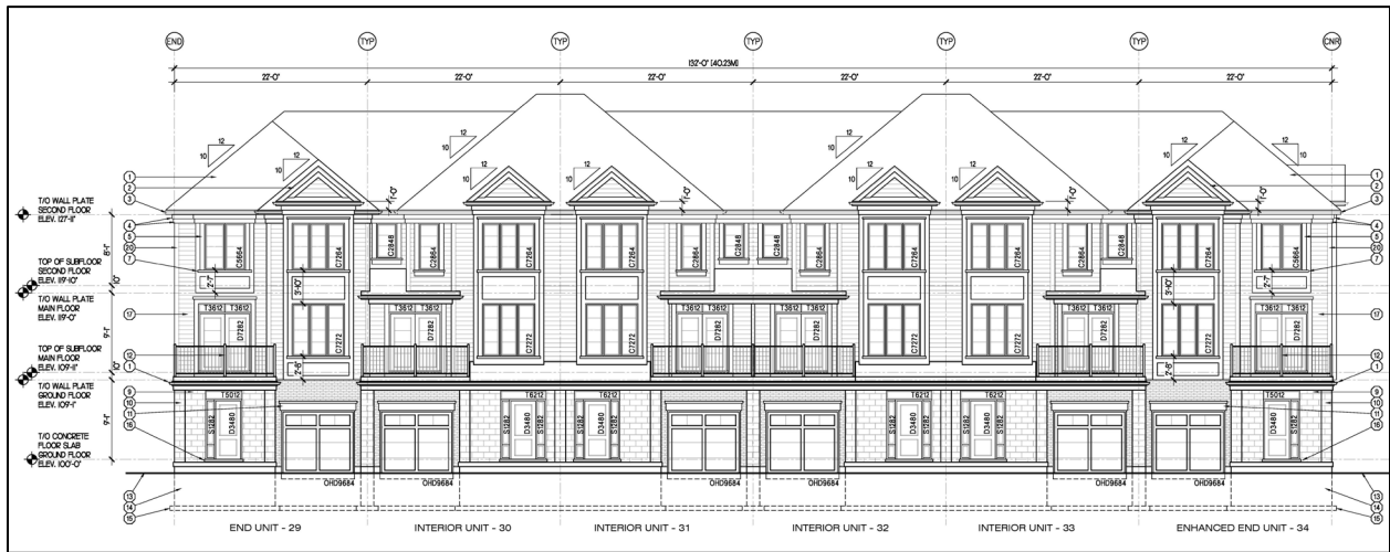
Figure 10 – Proposed Three-Storey Back-to-Back Townhouses Elevation (excerpt)
