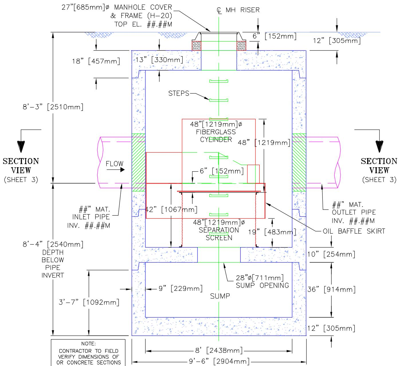
CDS MODEL PMSU40\_30m, 4.5 CFS TREATMENT CAPACITY
