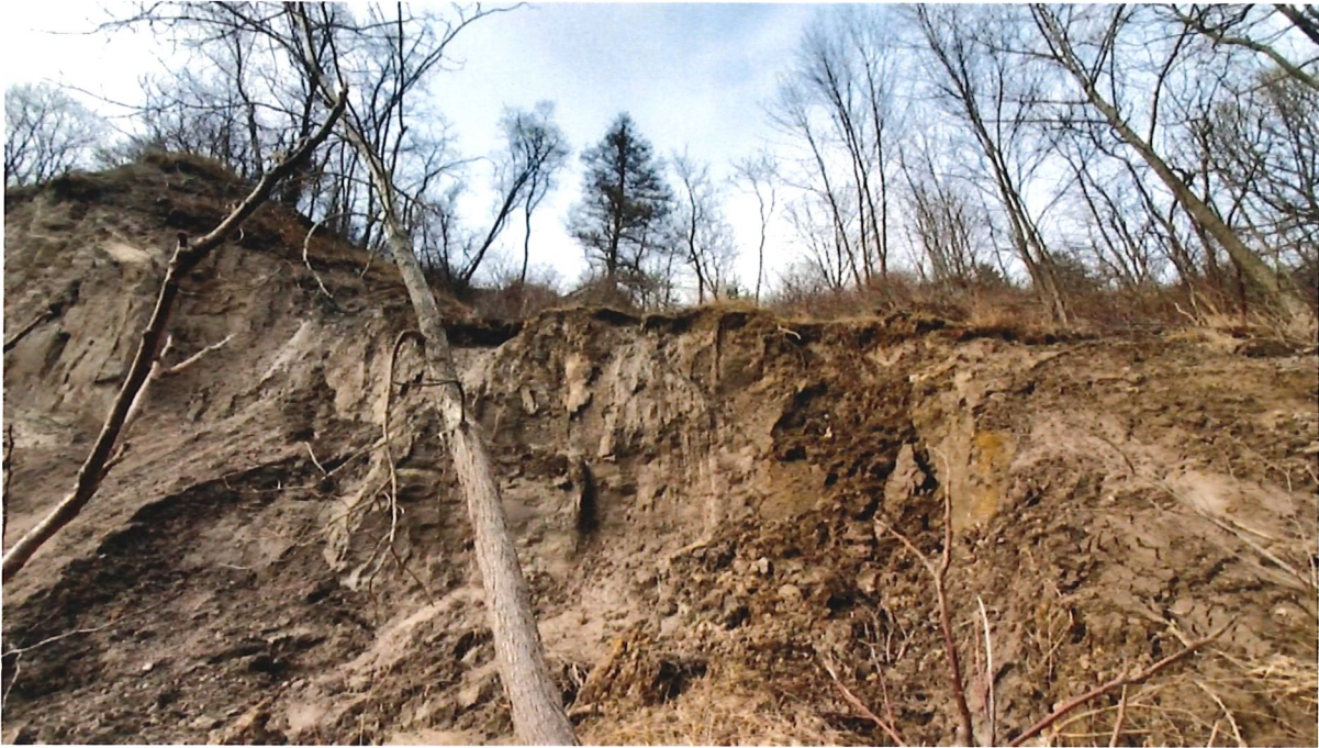
West side of ravine showing top of bank slope failure not related to flow in bottom of gully
